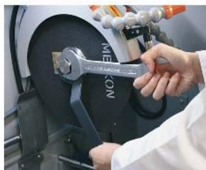
Easy Exchange of Cut Off Wheel
