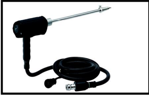
Industrial probe for interchangeable probe tubes with 9' or 16' sampling line and heated probe handle and easy replaceable quartz glass wool filter Available with and without heated sampling line
