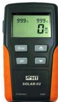
With **SOLAR-02** remote unit the irradiance and temperature measured values are shown at display also in independent mode (ideal solution during a pre-test on installation) besides test/recording with **SOLAR300N**
