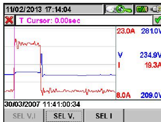
Fig. 128: Inrush currents graph
