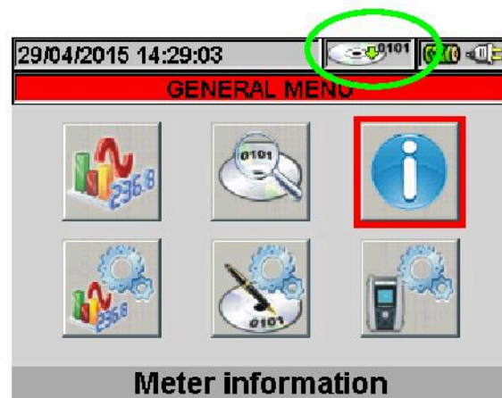
Fig. 106: Meter in recording run
