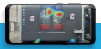
State-of-the-art machine tools exhibit a wide variety of complex sound events during the machining process. Engineers working in product development trust in the visualisation of sound radiation in order to take quick and effective measures to comply with noise limits.
