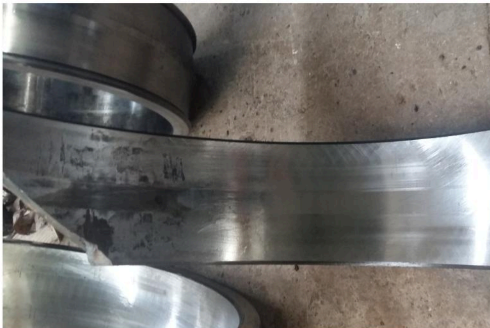
Image 3. Outer race bearing damage.
