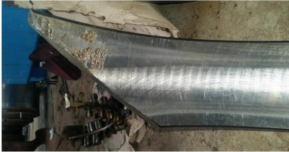
Image 4. Outer race damage.
