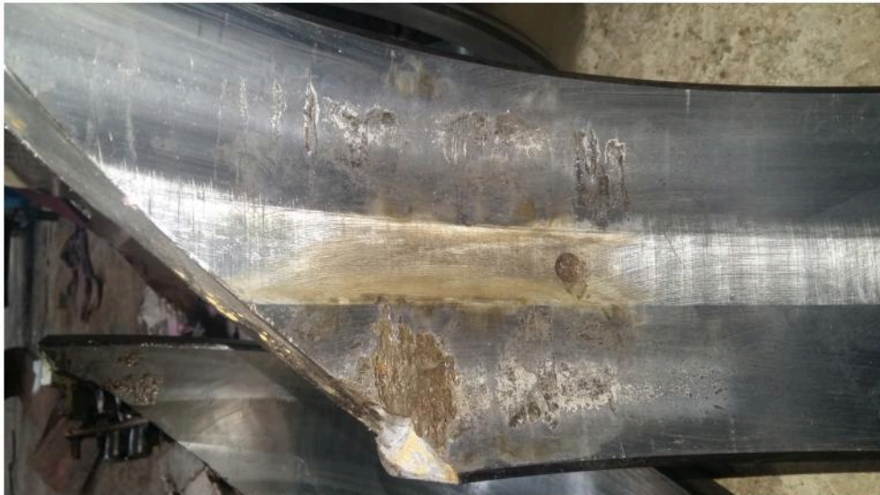
Image 2. Damage to the bearing outer race.
