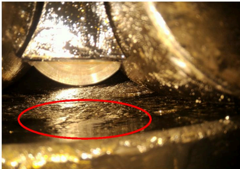
Image 3. Outer race damage.
